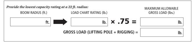
NOTE: Gross Loads used must be less than Maximum Allowable Gross Loads calculated above.
