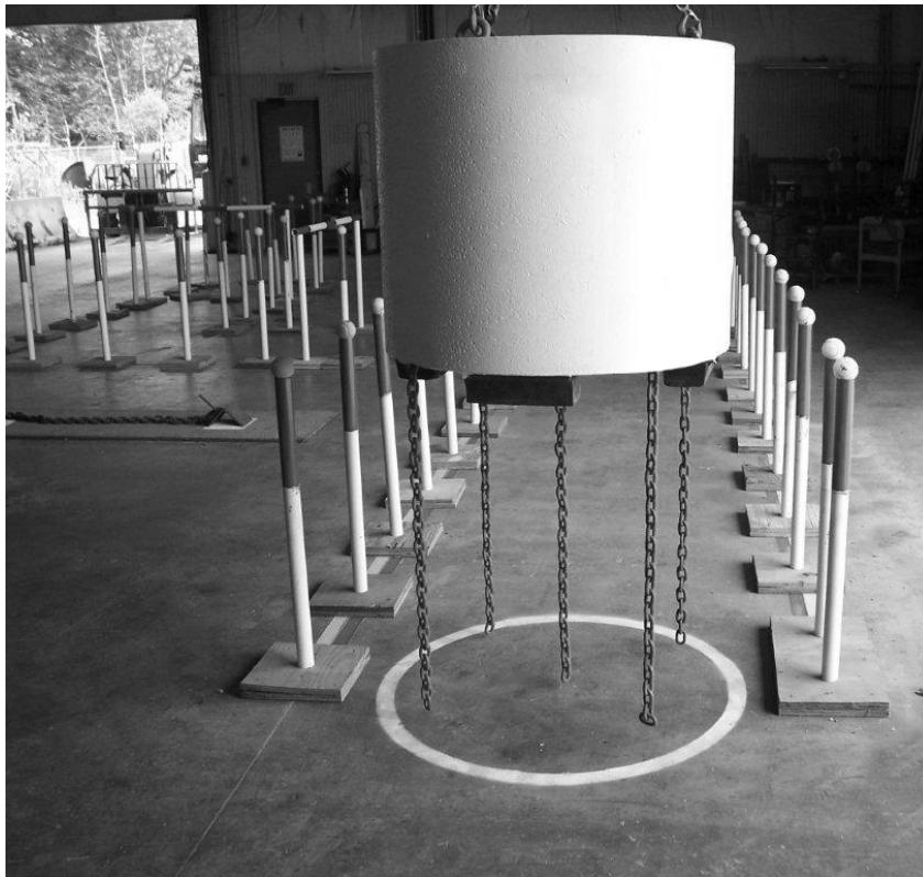
Test Weight with four additional perimeter chains (for cab-operated cranes with cab floor more than 25 ft. above ground only)
