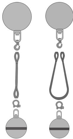
Rigging options for second overhaul ball
